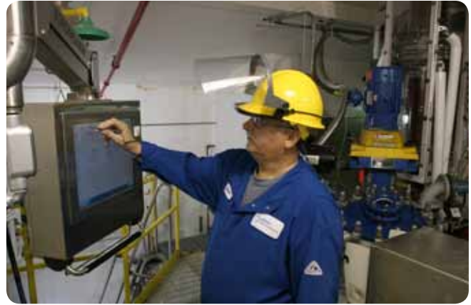
With the PlantPax system, plant operators at AFC enjoy decreased reliance on manual, paper-based batch sheets, thanks to an automated solution embedded directly into the control system.
